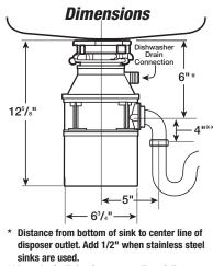
\*\* Length of tailpipe from center line of disposer outlet to end of tailpipe.
